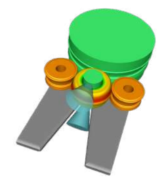
Ring rolling with temperature evolution
